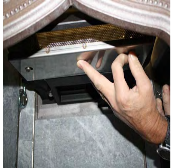
Scoop plate is sandwiched between the top roll pin and the cotter pin.
